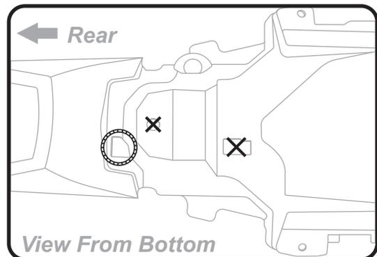
6. Re-connect the stock license plate light and turn signal connectors. Route wires in stock location and secure using supplied cable ties.
