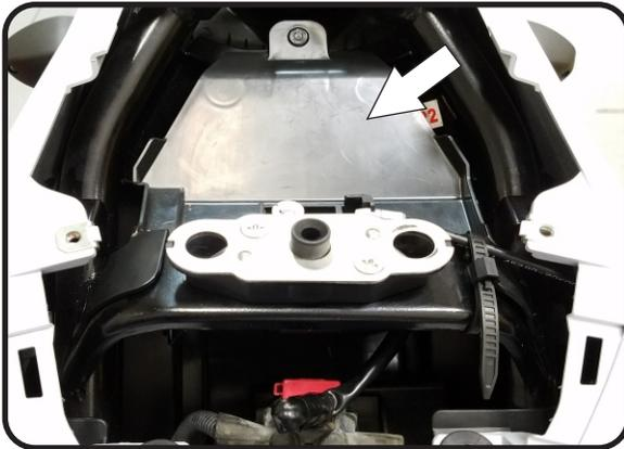
2. Disconnect the license plate light and turn signal wires.
