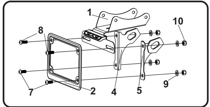
4. Route the wires from (No.3) *070BG-LH-K1*, licence plate light up through the hole in (No.1) *12202-FEBKT*, fender eliminator bracket.
