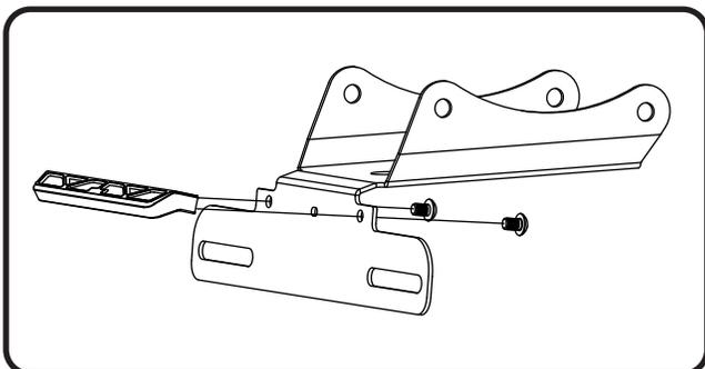
2. Install stock left and right turn signals onto (No. 4,5) *12202-TSB-L/R*, turn signal brackets using stock hardware.
