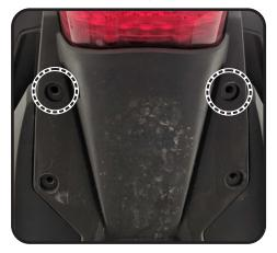
Note<sup>2</sup>: Spacer mounts between the undertail and fender bracket.
