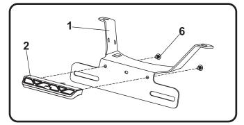
Route license plate light wire through hole in bracket and using the BN-SSS-22-18, solder shrink connectors supplied in the kit, connect Yoshimura license plate light wires to the stock license plate light wires as follows:
