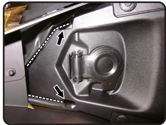
9. Re-install rear under-cowl and upper cowl using the opposite steps of removal.
