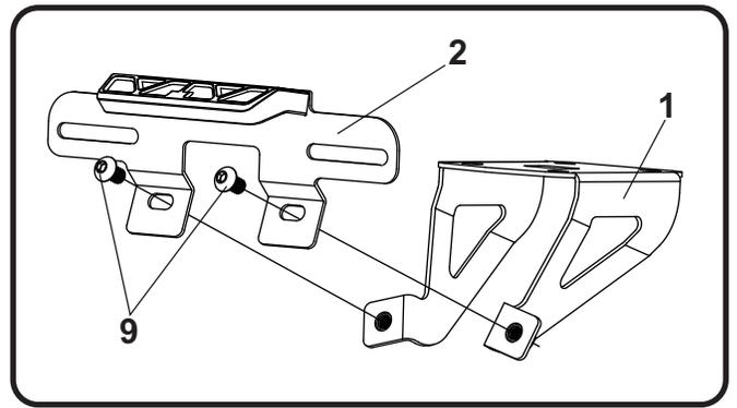
4. Assemble and install (No. 3) *070BG-LPF*, license plate frame and (No. 5,6) *14200-TSL/R*, left and right turn signal brackets onto (No. 2) *12200-FEBKT*, license plate bracket as shown.
