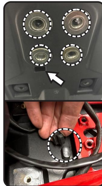
5. Route license plate light wires through loops on (No. 1) 19135-FEBKT, fender eliminator bracket and through hole in undertail where the rubber cover was previously removed.
