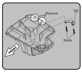
3. Install *HT SHLDR77*, muffler clamp heat insulator onto (No. 3) *YM7M-MPCAX*, muffler clamp.
