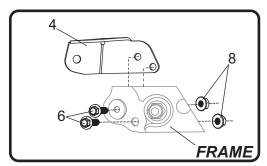
Remove the two right-rear oil pan bolts and install (No. 10) 13990-TPBKT, tailpipe bracket using the stock oil pan bolts. See assembly diagram for proper orientation of the tailpipe bracket. Torque oil pan bolts to 10 Nm (1.0 kg-m, 7.2 ft-lb).
