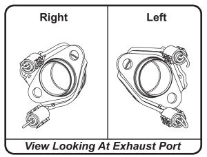
4. Install (No. 1) 22843-104/704, left header into manifold and hook (No. 9) RACE-SPX-1, small exhaust spring onto header using ST-200, spring puller tool supplied in the kit.
