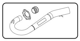
3. Install manifold and flange using the stock header nuts. Torque evenly to factory specifications.
