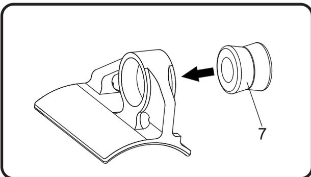
4. Install (No. 8) ALS-001, aluminum spacers into (No. 7) 011257-00, rubber bushings as shown. See assembly diagram for proper orientation.
