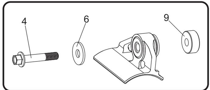
6. Torque (No. 4) M8X45H, bolts to factory specification.
