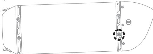
8. Remove adhesive backing and align nameplate rivet holes. Install new nameplate using the supplied nameplate rivets.
