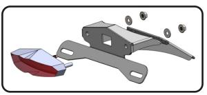
2. Install *H-2158,* wire cover into *11720-FEBKT,* fender bracket.
