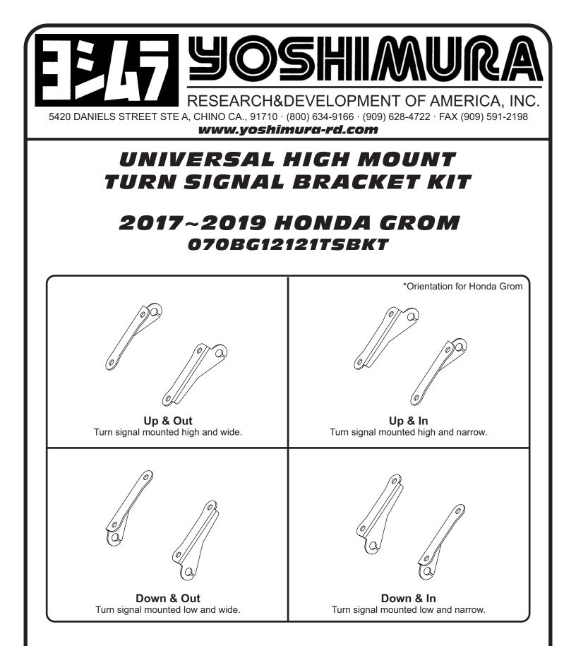
The Yoshimura Universal Turn Signal Brackets are to be used with aftermarket turn signals and can be installed using four different configurations. To prevent damage to turn signals, verify that the exhaust gases are not directed toward the turn signals. Yoshimura R&D of America, Inc. is not liable or responsible for any resulting event caused by the installation of this product. Check with local laws and regulations for compliance prior to installation and use.
