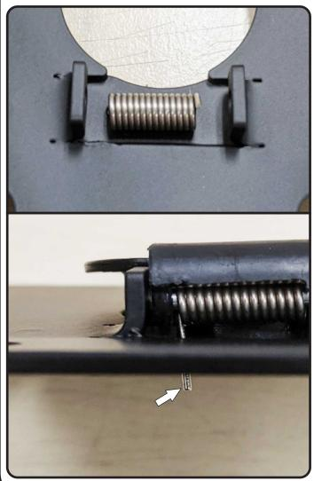
5. Locate the stock spring tension location on the key cover cap as shown in the diagram.
