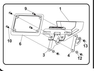
Install assembled fender eliminator bracket using (No. 11) *M6X30*, 6mm hex head bolts, (No. 12,13) 6MMWASHER and 6MMLN, washers and nuts.
