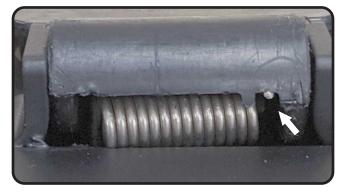
6. Have the OEM pin nearby to get ready for installation. Slide the key cover over the spring and keep pressure on the spring and cover.
