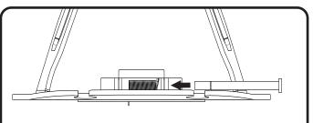
6. Slide the (No.14) *13992-FEBKTSPCR,* pin spacer onto the OEM pin and then install the stock circle clip.
