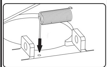
Note: The spring needs to sit flush with the fender eliminator bracket. Place the bracket on a flat surface and lift it.
