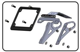
6. Install assembled fender eliminator using the stock fender bolts, *14720-SPR*, fender bracket spacer, and *8MMNUT*, 8mm flange nuts. Route license plate light and turn signal wires through *H-2158*, wire cover on fender eliminator bracket and through undertail. Torque bolts to factory specification.
