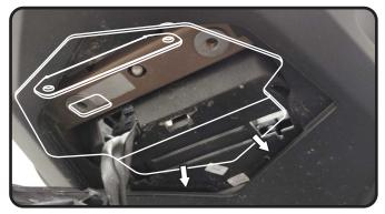
Install (No. 3) 070BG-LH-K1, license plate light onto (No. 2) 15204-FEBKT-2, license plate bracket using (No. 9) M4X6BHS, 4mm screws.
