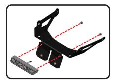
2. Install *FE-LP-BKT*, license plate bracket onto the fender eliminator bracket using *M6X12FS-SS*, flat head screws.
