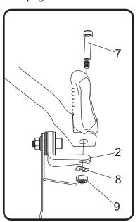
Standing at the back of the motorcycle, check and adjust muffler and bracket until desired alignment is achieved. Using a marker, mark (No. 2) 11100-BRKT, muffler mount bracket and (No. 1) muffler bracket.
