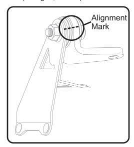
Repeat Step 5 and secure (No. 2) 11100-BRKT, muffler mount bracket to the right passenger footpeg bracket. Apply thread lock onto shoulder bolt threads.
