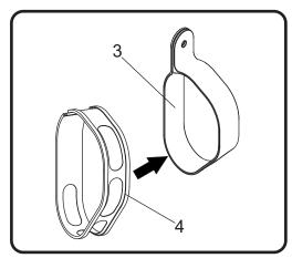
4. Slide (No. 3) MCYM5-GCBX(-X), muffler clamp over (No. 2) Muffler.
