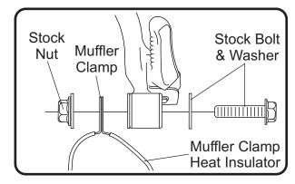
5. Install (No. 2) *Muffler* onto (No. 1) *11800-435*, tailpipe outlet. Align and secure to the stock muffler mount using the stock bolt, washer, and nut.
