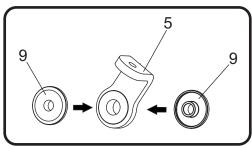
5. Install (No. 4) *HT SHLDR77,* muffler clamp heat insulator onto (No. 3) *MCYM5-GCBX(-X),* muffler clamp.
