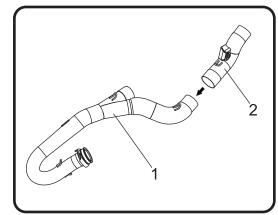
3. Install (No. 3) 22583-145/745, Yoshimura right tailpipe by sliding onto right header outlet. Align tailpipe chassis mount bracket to subframe and secure using the stock chassis mount bolt. Do not torque at this time.
