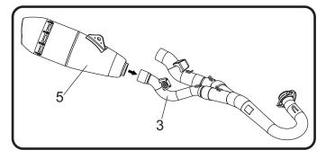
Install (No. 4) *left muffler*, over (No. 2) 22583-144/744, left tailpipe outlet. Align muffler mount bracket to muffler mount and secure using the stock muffler mount bolt and washer. Do not torque at this time.
