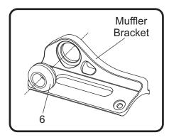
Install (7) ALS-003 aluminum spacer into (6) Z1022 rubber grommet as shown in the diagram.
