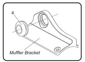
2. Install (No. 5) *ALS-040*, aluminum spacer into (No. 4) *Z1022*, round rubber grommet as shown.
