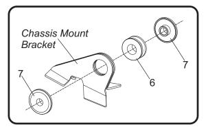
4. Install (No. 6) *Z1022*, rubber grommet into muffler resonator bracket as shown.
