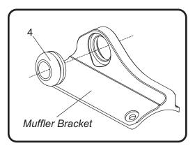
2. Install (No. 5) *ALS-002*, aluminum spacer into (No. 4) *Z1022*, round rubber grommet as shown.
