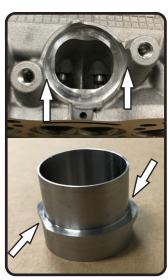
For 2005 ~ 2006 Suzuki engines the installation of the manifold to the cylinder head is critical to ensure proper alignment and seal.
