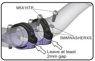
5. Torque the four clamp base bolts to 10 Nm.
