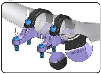
6. Torque the two forward clamp bolts to 5 Nm.
