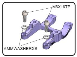
3. Grease 6mm x 35mm bolts and using 6mm washers install handlebar and upper clamps. Do not torque at this time.
