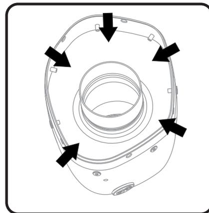
3. Re-install endcap assembly and align rivet holes.
