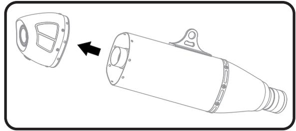
4. Remove baffle and clean carbon buildup. Inspect stainless steel mesh wrap on baffle.
